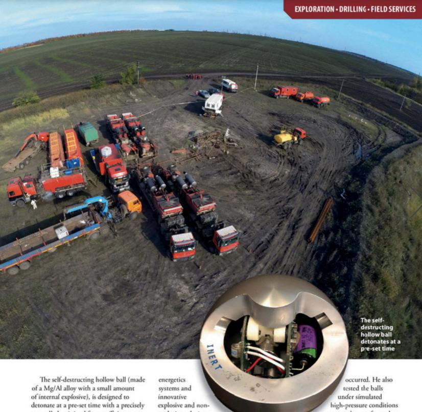
controlled, minimal force sufficient to break the ball apart and not damage the plug or surrounding casing. The remaining fragments are water soluble and will dissolve in two to three days.
